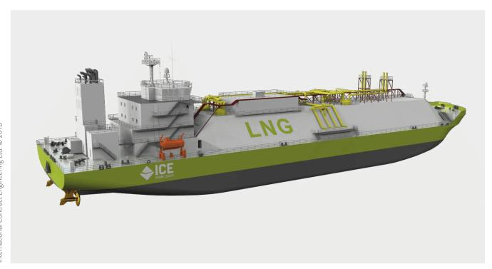
The type C bi-lobe cargo tanks have been dimensioned to maximize cargo-carrying capacity within a given set of hull dimensions and draft restrictions, without altering the ship's performance.
