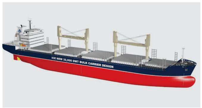
She is laid out with 5 cargo holds and equipped with four 30 tonnes SWL deck cranes (holds 2, 3 and 4 are fully box shaped and holds 1 and 5 are semi-box type with lower hopper slopes as necessary to provide double skin).
