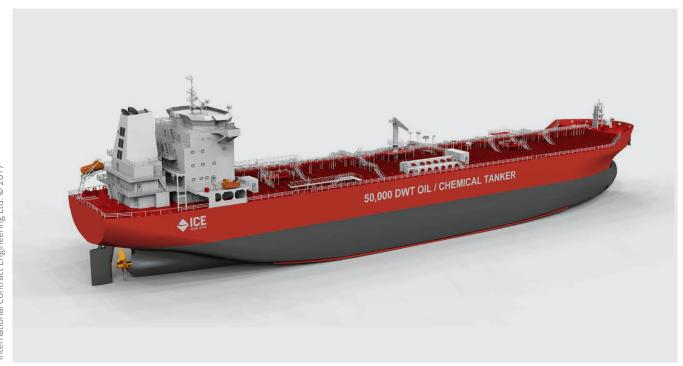
The vessel has been developed in accordance with the relevant HCSR and IMO regulations. She is a single screw motor tanker with low speed engine and high propulsion efficiency and has 12 cargo tanks, each equipped with submerged cargo pumps, plus 2 slop tanks and 1 retention tank. The ship will be fitted with a Tier III main engine, including EGR (exhaust gas recirculation), EGCS (exhaust gas cleaning system) and SCR (Selective catalytic reduction).
