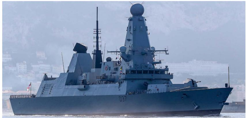
Length overall: 152.4 m, Beam: 21.2 m, Draft: 7.4 m, Displacement: 8,500 tons
